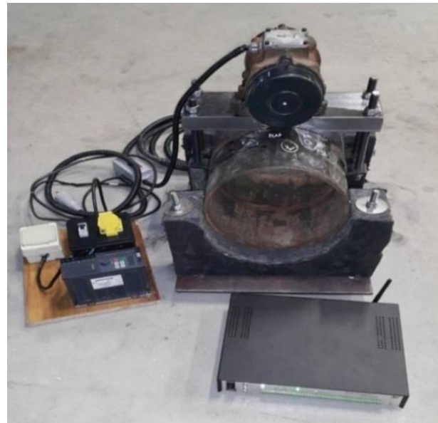
Fig. 3 Vibration stress relief setup on pipe
